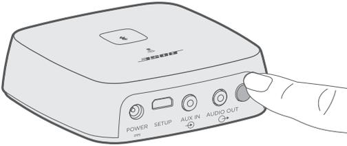
2. When the Wi-Fi indicator turns off, release the **Control** button.
